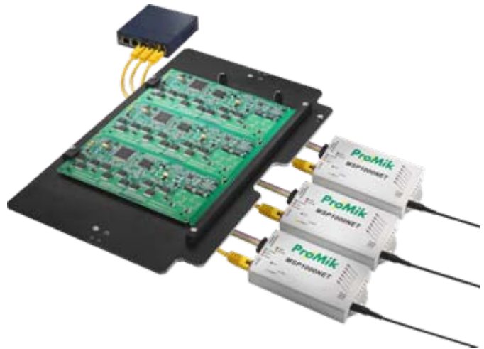
Parallel programming, PCB on a bed-of-needles adapter
